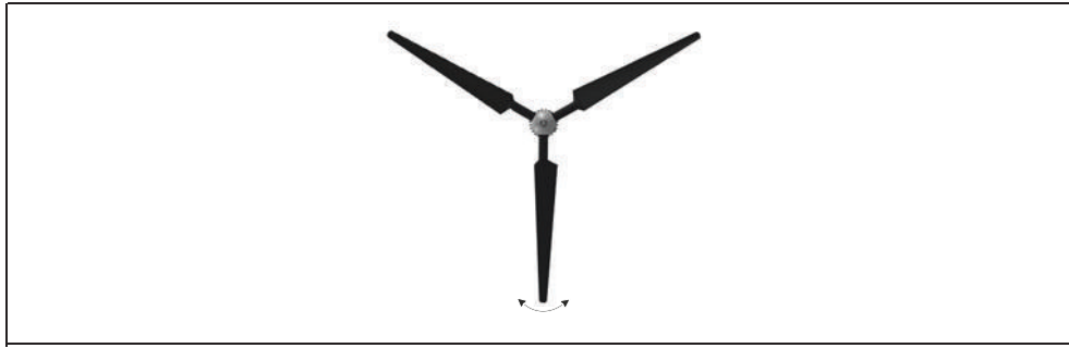
Fig. 7: Balancing the rotor (Y position)
